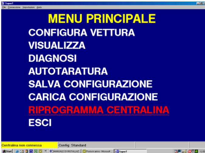
Select RE-PROGRAM ECU from the main menu and press Enter. This menu is used if you should need to re-program the control unit following an up-date of the “Firmware” on behalf of Tartarini Auto, for improvement purposes or to add new program functions.
