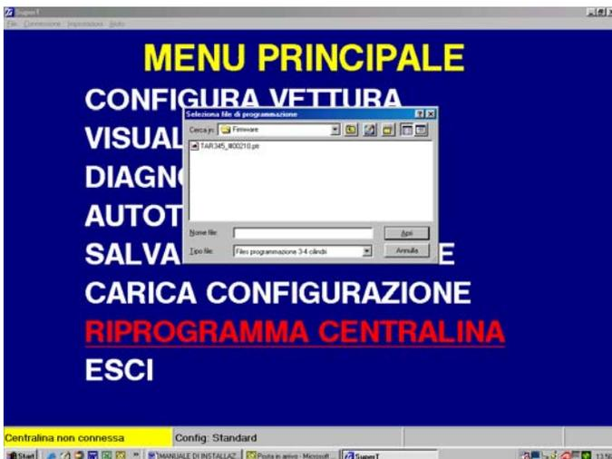
To be able to program, select the file containing the new “Firmware” for the control unit, through a communication window. Once you have selected the file, simply click on the Program tab to start up-dating the control unit.
