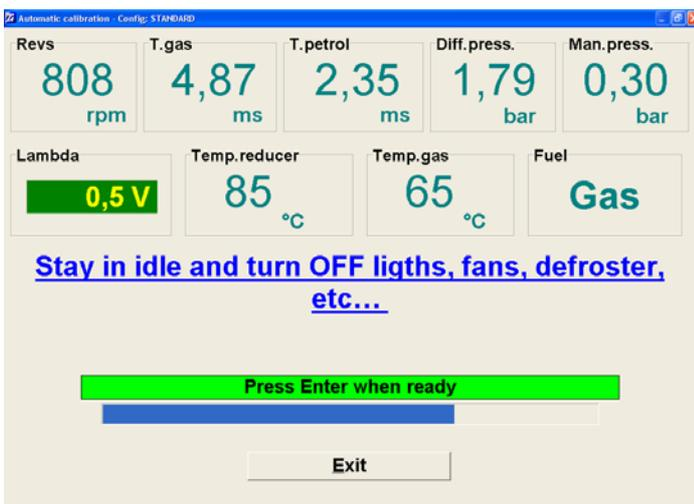
Leave the engine running at minimum without acceleratine, turn the lights and the demister off and wait a few seconds before pressing ENTER.
