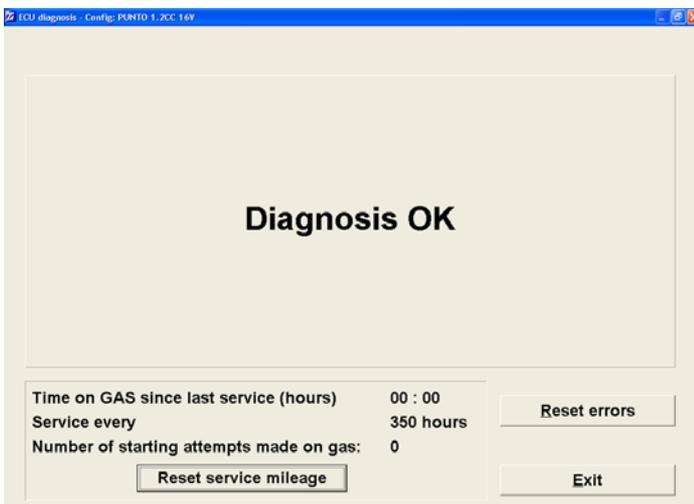
If there are no errors in the controller, the page appears as illustrated. If on the other hand an error is detected, the type of error will be indicated with the possibility to cancel it using the **reset errors** button.
