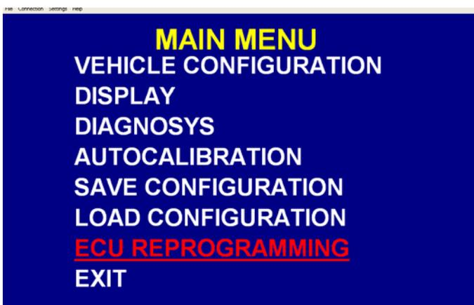
Select RE-PROGRAM ECU from the main menu and press Enter. This menu is used if you should need to re-program the control unit following an up-date of the “Firmware” on behalf of Tartarini Auto, for improvement purposes or to add new program functions.
