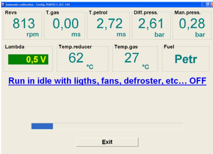
The system will request you to leave the engine running at minimum with all the vehicle's accessories switched off.
