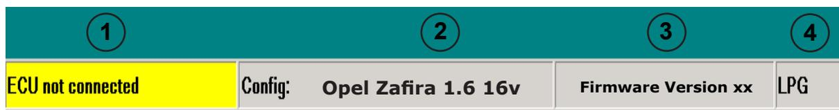
1) indicates whether the control unit is connected or disconnected to the calibration software. It is important to remember that all the settings made on the disconnected control unit will be lost when it is connected, unless they are previously saved in a configuration file.
