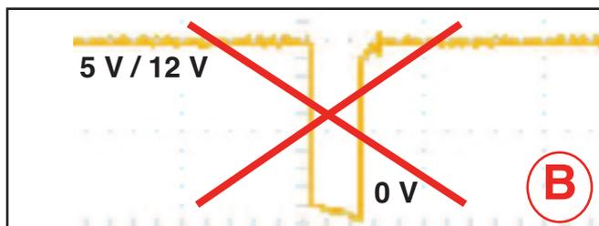
**CASE B** Low voltage coil signal. Vehicle **CAN NOT** be converted with P&D SCORPIO
