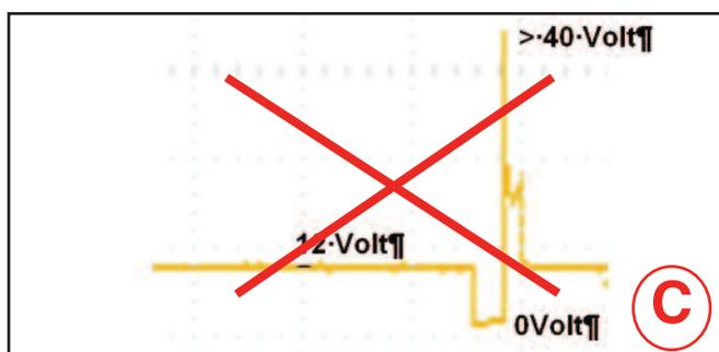
**CASE C** High voltage coil signal. Vehicle **CAN NOT** be converted with P&D SCORPIO
