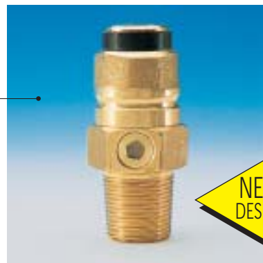
66.0241 66.0.290.0241 "Jumbo" valve with fusible plug. Valve designed to be used with the new technology cylinders in composite and/or aluminium materials. 28,8 x 1/4" DIN 477 inlet. With pressure relief device.
