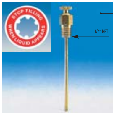
66.1072 66.0.290.1072 Fixed liquid level gauge. Available with different dip-tube lengths. An optional instruction plate may be ordered for use with these valves.
