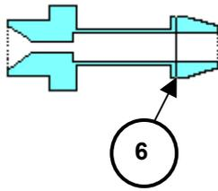
The reference marks that identify the type of nozzle to be used can be seen on the outer edge of the nozzle, as illustrated in fig. 6.
