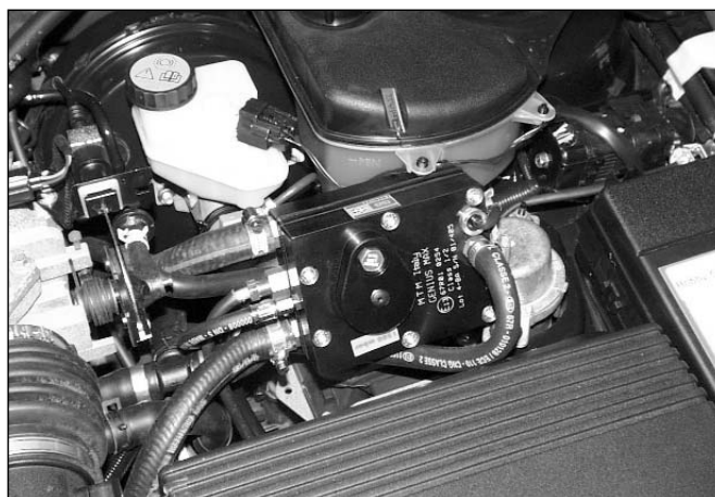
Picture 04 LPG Sequent Genius MAX: possi- ble installation posi- tion
