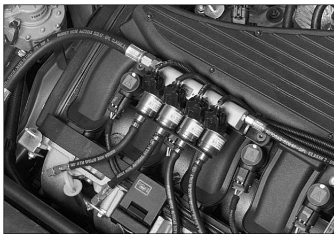
Picture 13 Example of the rail installation with Keihin injectors
