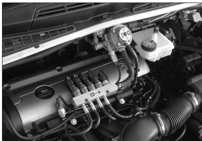
Picture 05 CNG Sequent Zenith Reducer: example of installation
