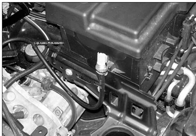
Picture 16 Example of the Sequent Fastness MAP sensor installation
