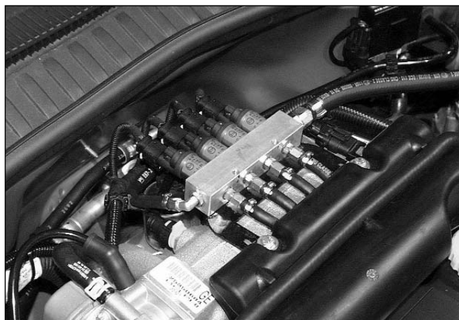
Picture 12 Example of the rail installation with BRC injectors
