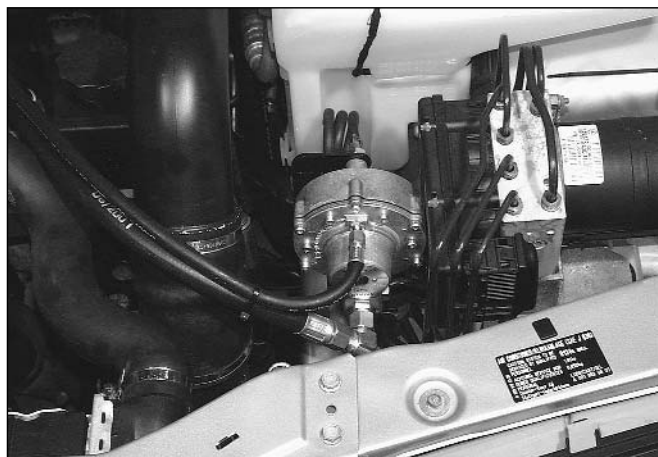
Picture 02 Sequent Genius reducer installation with diaphragm per- pendicular to the driving direction
