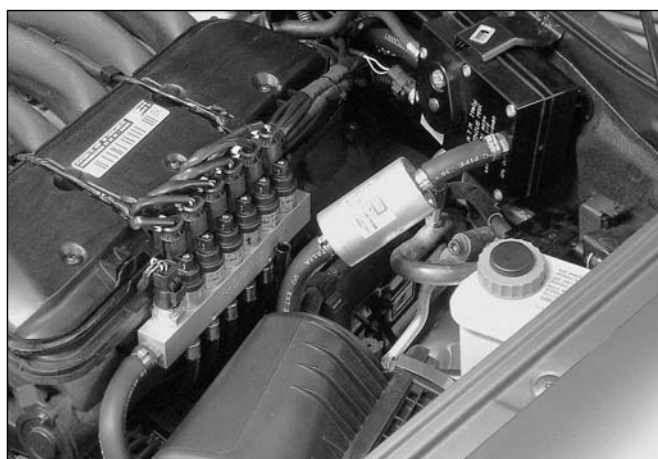
Picture 14 Example of the rail installation with BRC injectors and temperature and pressure sensor gas
