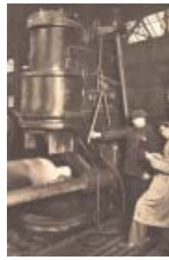
Forming of the tube end The fifties
